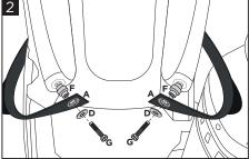
Place the bushings (F), the strap (A), the washers (D) and tighten using the screws (G). Inserire le boccole (F), cinghia (A), rondelle (D) e avvitare tramite viti (G).
