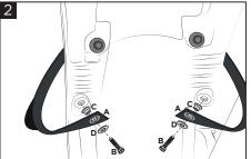
Place the bushings (C), the strap (A), the washers (D) and tighten using the screws (B). Inserire le boccole (C), cinghia (A), rondelle (D) e avvitare tramite viti (B).
