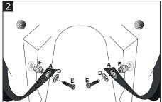
Place the bushings (F), the strap (A) the washers (D) and tighten using the screws (E). Inserire le boccole (F), cinghia (A), rondelle (D) e avvitare tramite viti (E).
